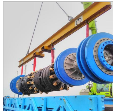
Figure 18 40in SmartPlug isolation tool before insertion
