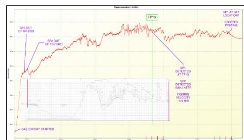
Figure 18 Recorded pigging pressure
