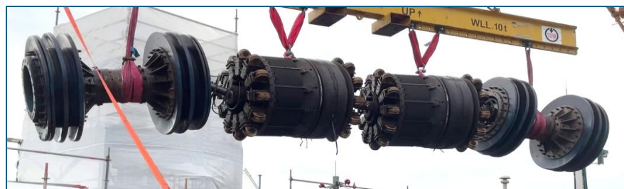
Figure 19 40in SmartPlug tool after 670km pigging
