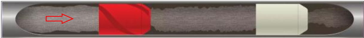
Figure 8 Foam Pigs moving through pipeline
