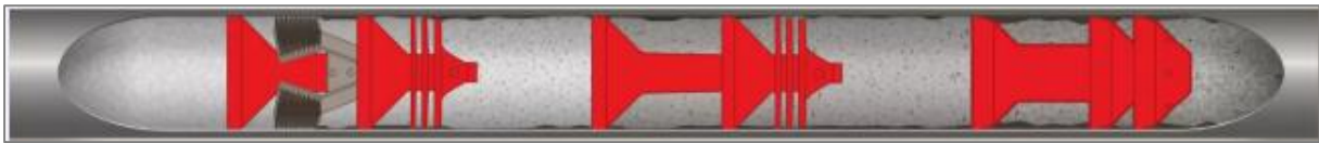
Figure 9 Pigs used to remove debris and content
